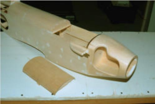
The kit is very complete with all necessary hardware and very good quality wood and a very detailed building manual. The kit is a combination of laser cut parts for the fuselage, die cut wing ribs and shaped
