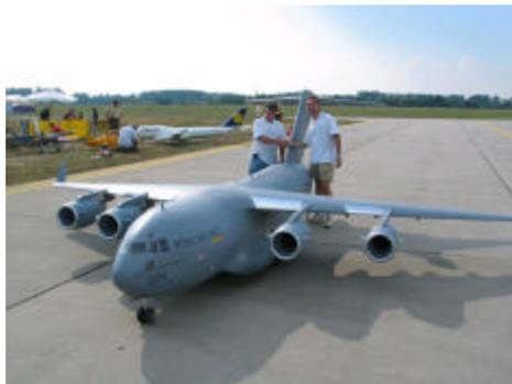
including airspeed, turbine RPM, EGT and fuel consumption, to a laptop computer on the ground. The model was built mainly from balsa and plywood, with many glass and carbon fiber moldings to reduce weight. It is covered in fiberglass and epoxy resin. This C-17 Globe Master III is one of the largest jet models in the world today.
