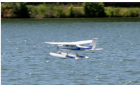
Landing is very straight forward as long as you keep the nose up as the plane slows. As lift melts away, the craft will just settle nicely onto the water and things will be fine. If you come
