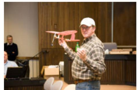
home designed and built electric. It was constructed from balsa sticks and covered with tissue. He powered this plane with an electric out-runner. He calls his model the "mist", a bigger version of the popular Vapor.
