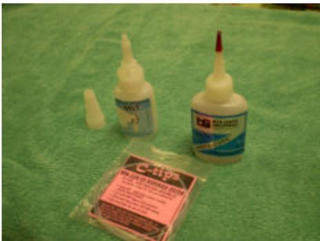
A bottle of the Mercury CA is shown on the left with the cap removed. The needle that pierces the opening is inside the cap. Note the stubby tip of the Mercury bottle which makes it hard to put the glue in tight places. A better solution is shown on the right with Teflon tubing attached to the tip of the bottle with a piece of shrink tubing.
