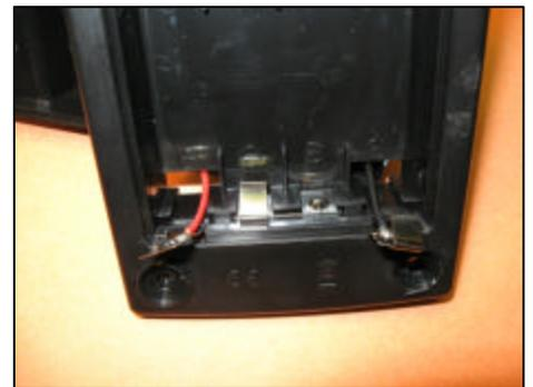
Next, we need to drill a hole in the bottom part of the case for the battery charging lead. You can either put the hole in the front or in the back of the case. I have done it both ways and prefer having it at the back. If you
