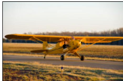
Empty weight is 710#; 65hp; gross weight is 1220#. It cruises at 68 mph (or so), stalls at 38, although I have flown it as slow as 30mph. 65hp is ok when it's cold out, but it requires a lot of fore thought on hot humid days. My bet is that your 50% cub has a higher power to weight ratio. Your photos look like a Reed clipped version.
