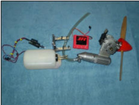
The following glow-related equipment was removed: Fuel tank, 40 2-stroke engine, prop and spinner, engine mount, receiver battery, switch, tail brace (not shown).
