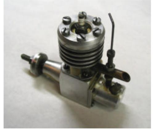
He also showed me a glow engine that he made from plans he saw in a magazine. He said that it did run but never put in an airplane. A nice piece of work as shown in one of the pictures.
