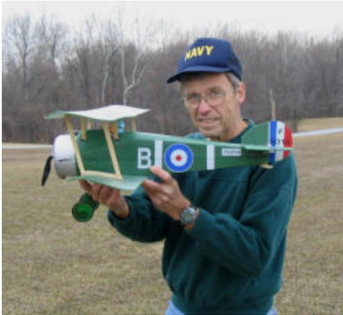
little more rudder through. I'm using the stock 370 motor, gear box and 10x5 prop which provide enough power for relaxing scale-like flying. The remaining onboard equipment includes a WattAge IC-5A ESC, two FMA S90 sub micro servos a GWS R-4P Rx and a 2 cell 830 mAh Tanic LiPo pack. It took 3/4 ounce of nose weight to balance, so I may trade up to a higher capacity battery pack at some point.
