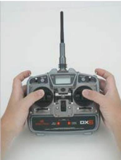
Because there are two antennas with different positions, if in the unlikely event a frame is dropped (loss of signal for more than 15ms), the other receiver is already on-line. Result: No interruption in signal. No dropouts. No problems. Just a strong, solid link. That's what DSM Dualink is all about.
