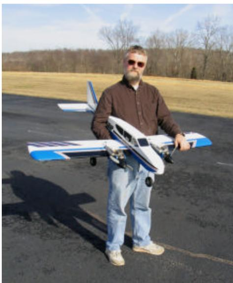
recently with a different sounding model- a Hobbico TwinStar. For power, Ed is using two OS 25FX's which pull it along nicely. He added access openings on each engine nacelle to make it easier to adjust the engine throttle linkage for better rpm synchronization. The model flies well but he did add some checker-board covering to the bottom of the wing for better visibility. Radio is a Futaba Skysport 4 with stock servos.
