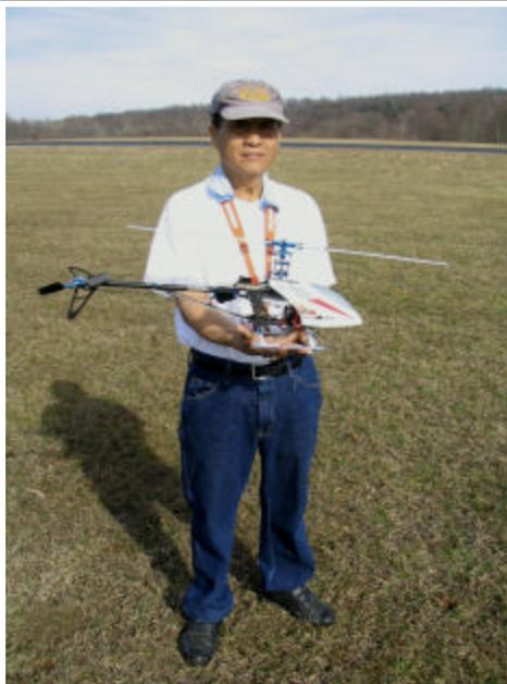
equipped with a Lener brushless motor and a Li ESC. The LiPo battery pack consists of three 2100 mAh Thunder Power cells in series. He is using a Futaba 14MZ radio and Hitec analog servos for everything except the tail rotor, which uses a Futaba
