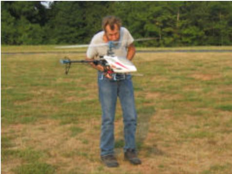
Align brushless motor and a Perlite 2100 3S Lipo battery. The flying weight is 720 gm. or about 25 oz. The model is equipped with a Futaba receiver and 401 gyro, and Hitec HS-56 servos. It is set up with Cyclic/Collective Pitch Mixing (CCPM). Average flying time is about 7 minutes.
