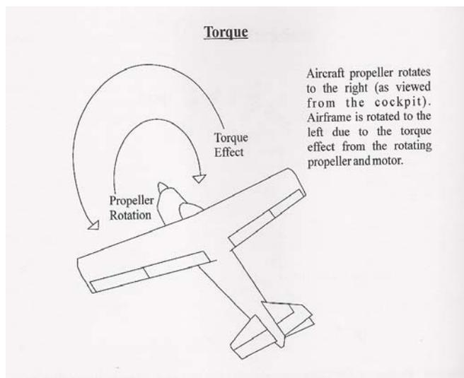
**Figure 6-1 Torque Induced Roll**
