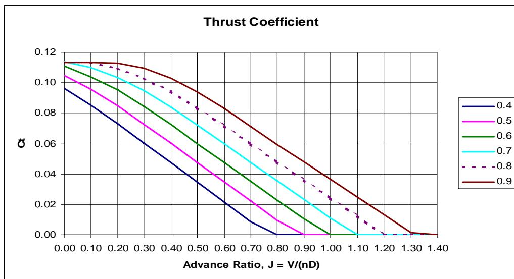
Figure 3-1. Thrust Coefficient Graph
