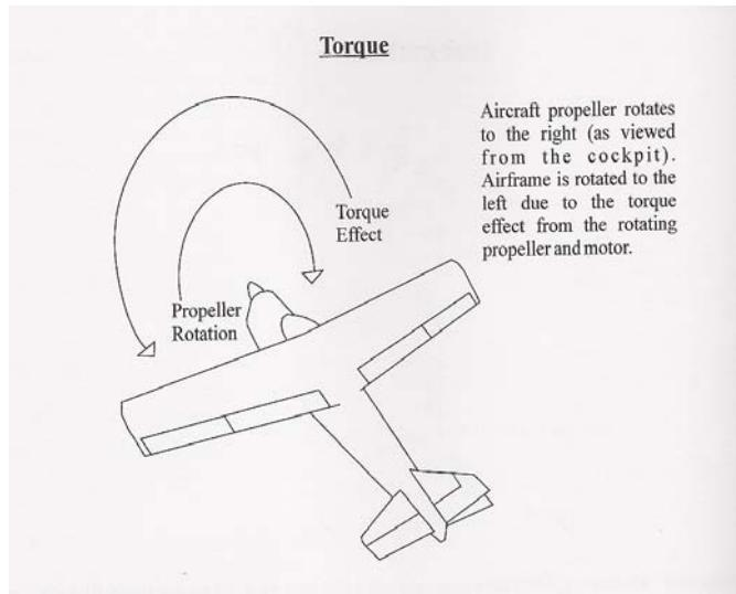
**Figure 6-1 Torque Induced Roll**
