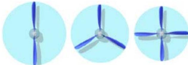
This figure shows the resulting relative size for 2, 3 and 4 - bladed propellers having approximately the same performance
