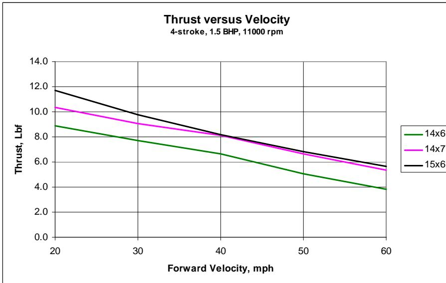
**Figure 4-4. Example Thrust versus Velocity Graph**
