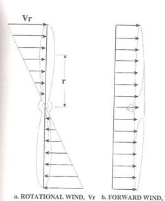
**Figure 2-2 Rotational and Forward Wind Vectors Along the Propeller**
