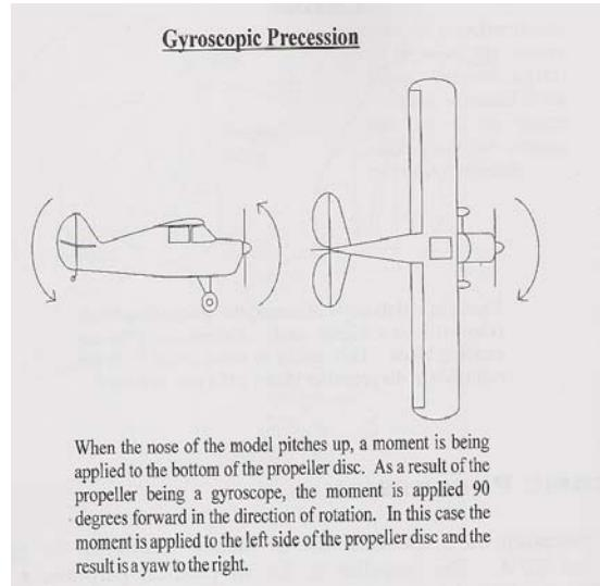
**Figure 6-3 Gyroscopic Precession.**
