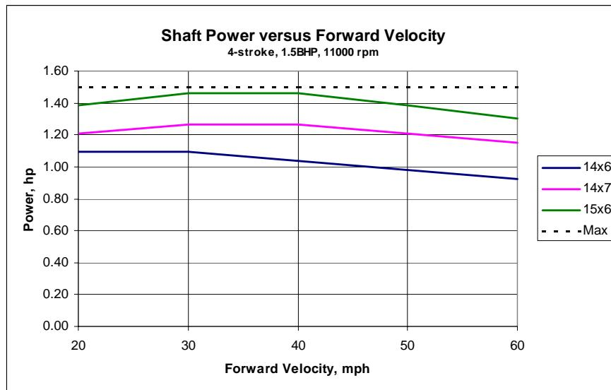
**Figure 4-5. Example Engine Power versus Forward Velocity**
