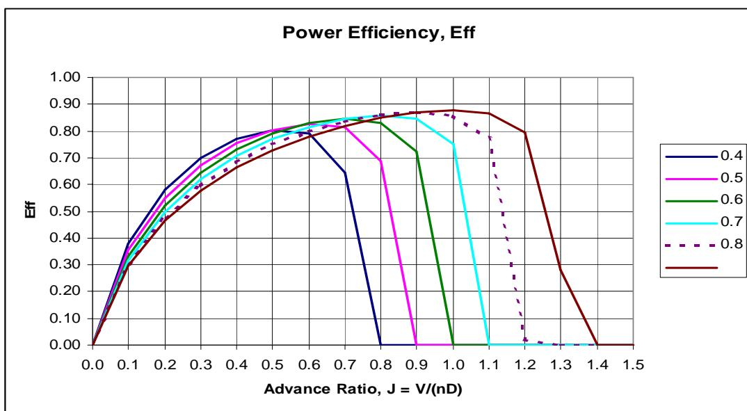
**Figure 3-3. Efficiency Coefficient**
