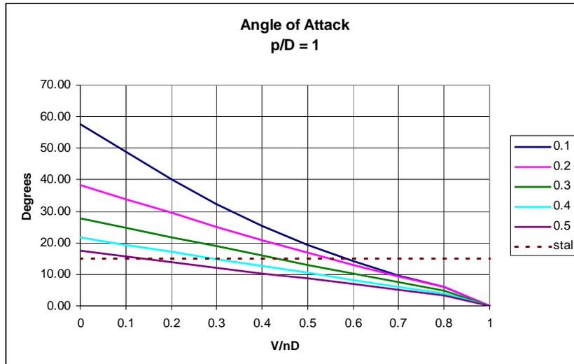
**Figure 2-5 Blade Angle of Attack,  $p/D = 1$**
