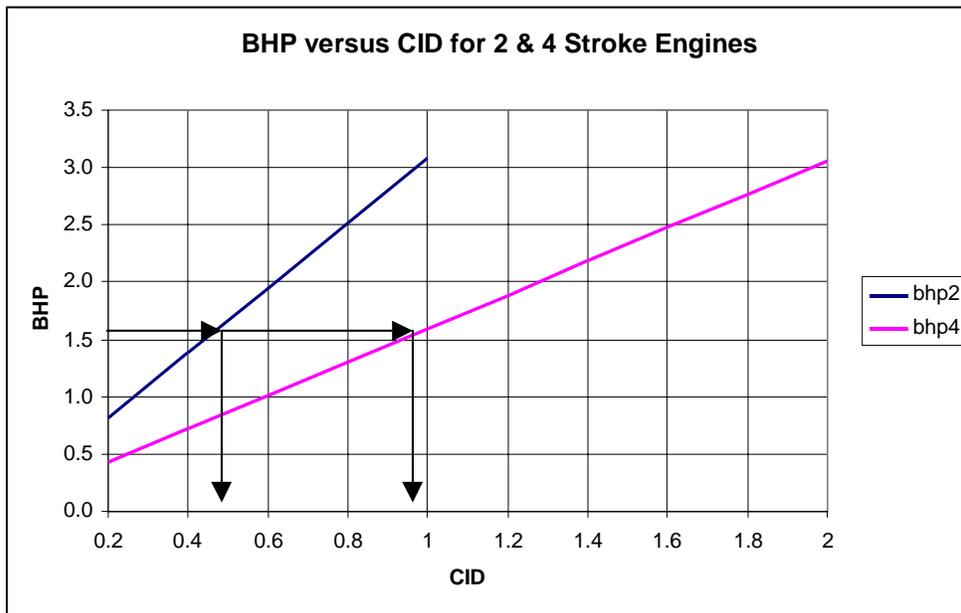
Figure 4-2. Relationship between BHP and CID for 2 & 4-stroke engines
