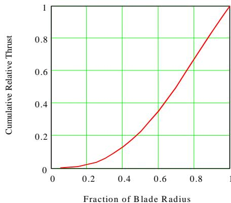
**Figure 1-3 Cumulative Thrust versus Relative Blade Radius**
