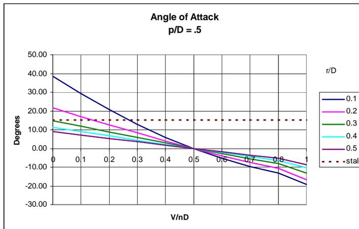
Figure 2-4 Blade Angle of Attack,  $p/D = .5$
