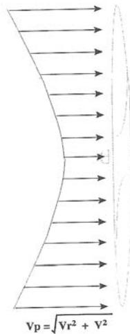
Figure 3.6 Propeller Wind.
