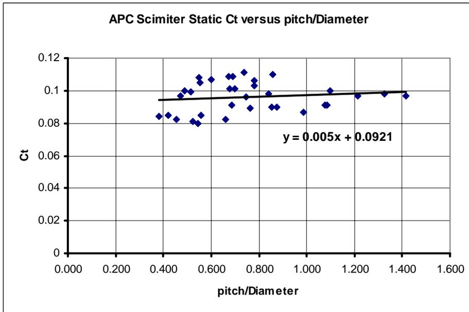
**Figure 5-2 APC Scimitar Static Thrust Coefficients**
