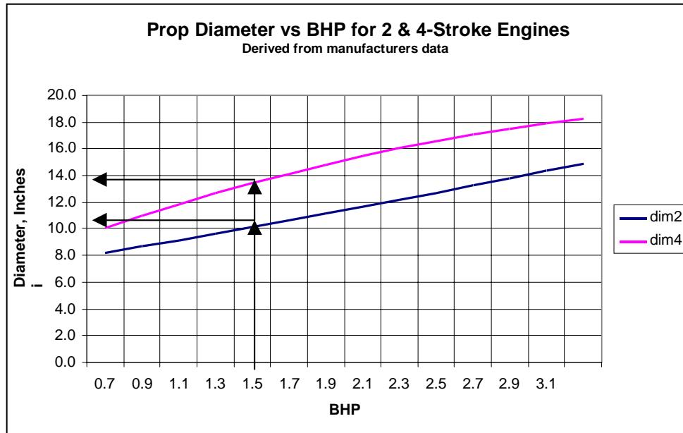
**Figure 4-3. Nominal Recommended Propeller Diameter for a Given BHP Requirement**
