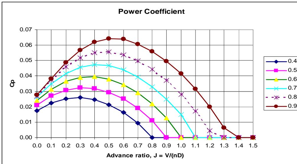
**Figure3-2. Power Coefficient versus Advance Ratio, p/D a Parameter**
