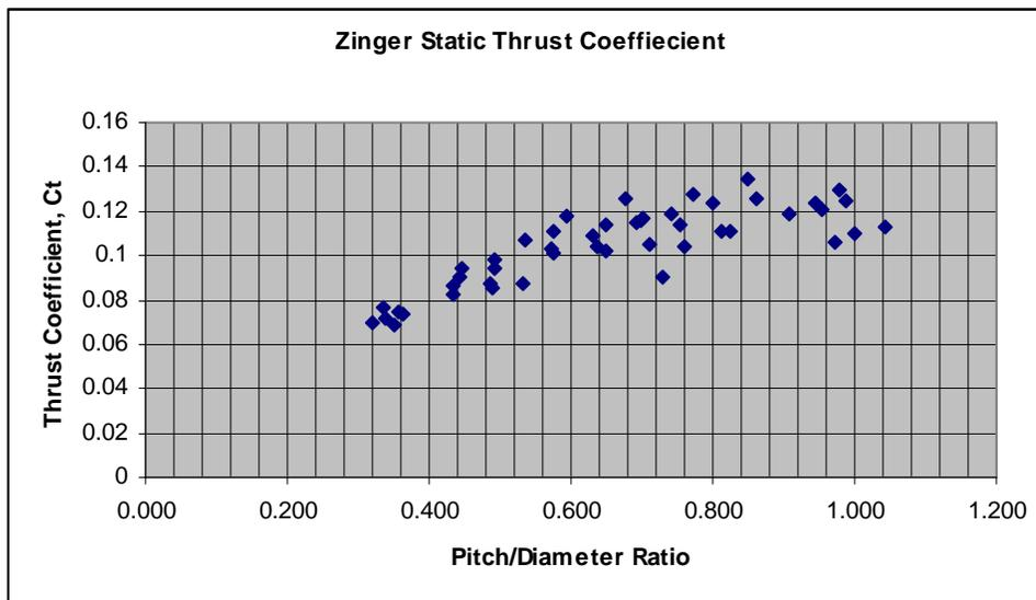
**Figure 5-1 Zinger Static Thrust Coefficient vs p/D Ratio**
