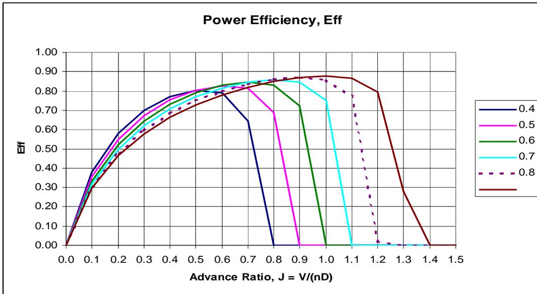
**Figure 3-3. Efficiency Coefficient**
