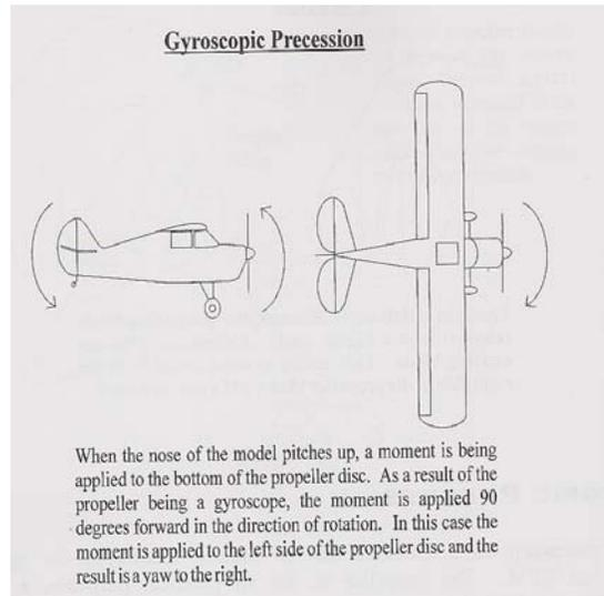
**Figure 6-3 Gyroscopic Precession.**
