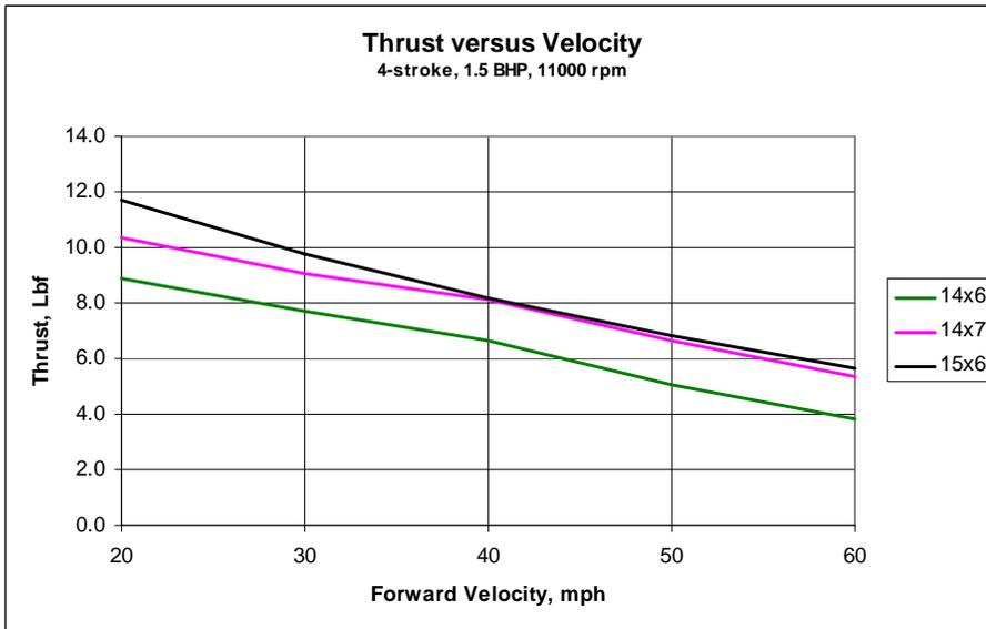
**Figure 4-4. Example Thrust versus Velocity Graph**
