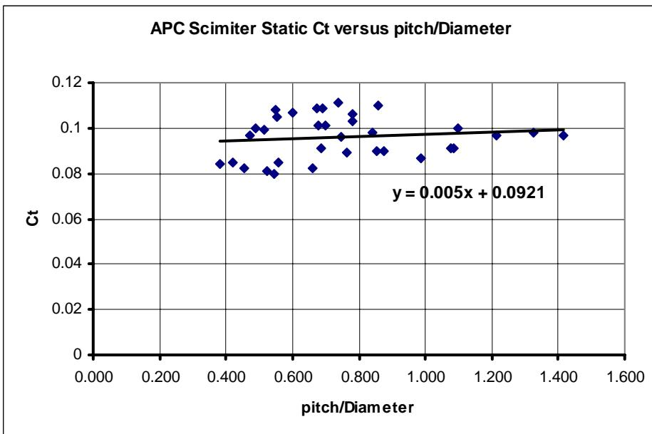
**Figure 5-2 APC Scimitar Static Thrust Coefficients**
