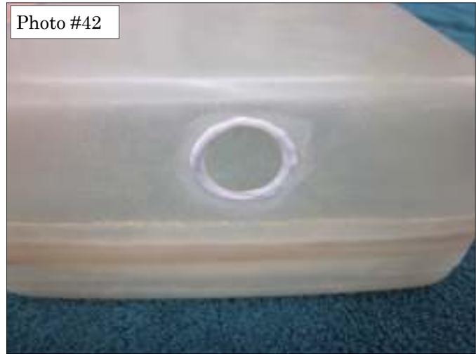
Open up the hole that you marked out before for the tapped hole to fit the MAP fittings for a snug fit. Scuff up the glass around this hole and wipe both the fiberglass and aluminum fitting with denatured alcohol. Apply a bead of Loctite/Hysol 9462 to the fittings glue
