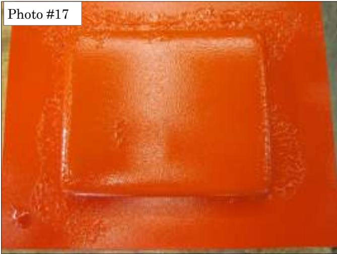
it too heavy the air pressure will blow the gel-coat around and cause it to ripple. Try to avoid this but don't panic if it does. (See photo # 17.)
