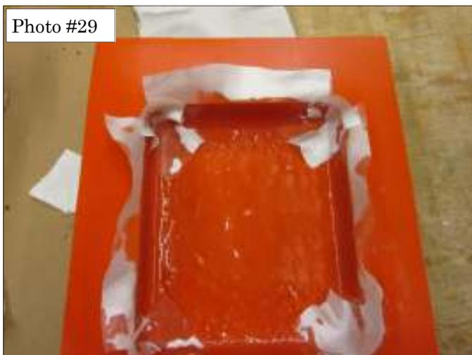
Now add the final layer of 3 oz glass the same way the first two were done. When you have all three layers and the corners in and have rolled out all the air pockets go back and use your 1 1/2 inch foam brush to dab any
