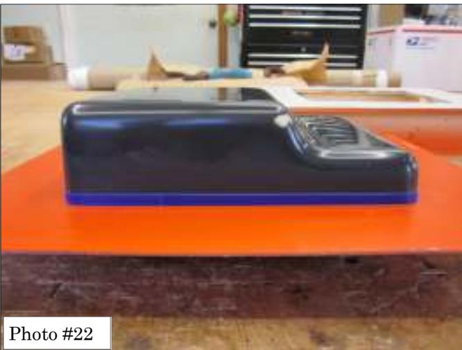
the entire surfaces as before. Cut the glass mat to necessary sizes for what was the parting board surface, plug sides and top. These can be one piece, even for an odd shaped mold like we are working with. They will
