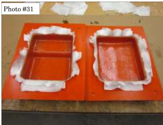
(See photos #30 & #31.) Now set them aside for the epoxy to set up a little. You want the epoxy to get to a sticky but firm condition so that we can trim the extra fiberglass from the tank halves before the epoxy sets up completely. When the epoxy has cured to a point where you can touch it and is sticky (but will not get your finger wet) it is ready to trim. Start with a new single edge razor blade and from inside the mold work the razor blade into the fiberglass layers flush with the mold (see
