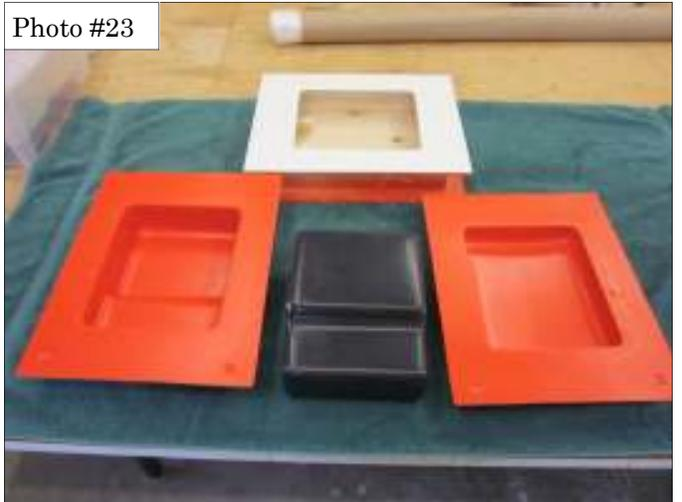
Lay the second layer just like before and let it cure overnight. Scuff the glass mat surface and apply the third and fourth layers as before and let them cure overnight. Trim the top of the mold to match the bottom and clean up the edges with sand paper. Now we get to separate the 2 mold halves. Gently work a screwdriver
