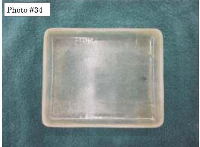
lightly and then wash all the release agent off with warm soapy water. The halves will not fit together without sanding the edges inside the tank. The corners will need the most work due to the small the small corner square during lay-up. Scuff up the and taper the outside edge of the tank without the indent so it will slide up into the other half with the indent. You will also need to sand the inside gluing lip area and the cor-
